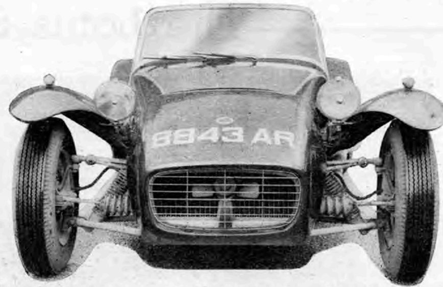
Nothing that isn't essential—though the lighting arrangements are not completely ideal for fast night driving. Note the electrically driven radiator fan which is controlled by a fascia switch.
