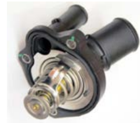
The thermostat controls a continuous circulation of coolant around the block - mixing between cooler radiator, and hotter bypass circuits.
