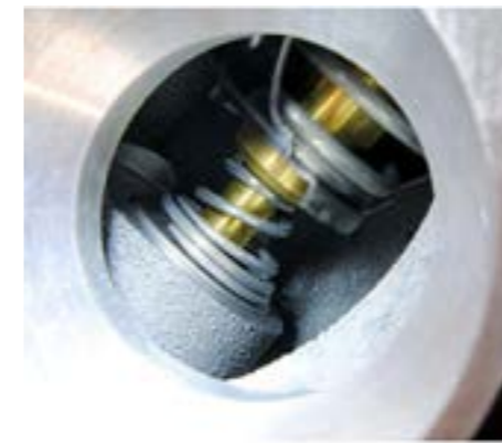
The thermostat controls a continuous circulation of coolant around the block - mixing between cooler radiator, and hotter bypass circuits.
