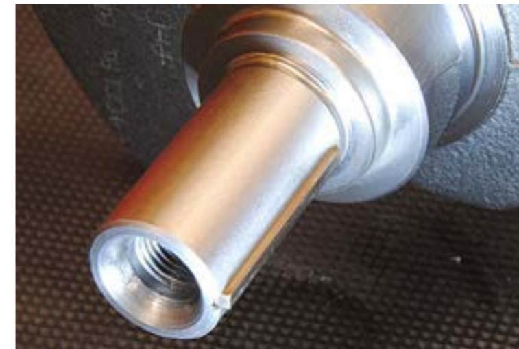
Die Keilnut muss das Ritzel einschließen, aber die Position muss stimmen. The keyway should include the pulley, but its relationship to the trigger wheel must not be forgotten
