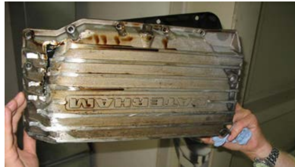
Schuld am Tod von KH-RC 120 I war ein Gullydeckel A gully cover was to blame for the death of KH-RC 120 I
